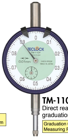
TM-110PW Oil-Proof type Graduation 0.01mm Measuring Range 10mm
